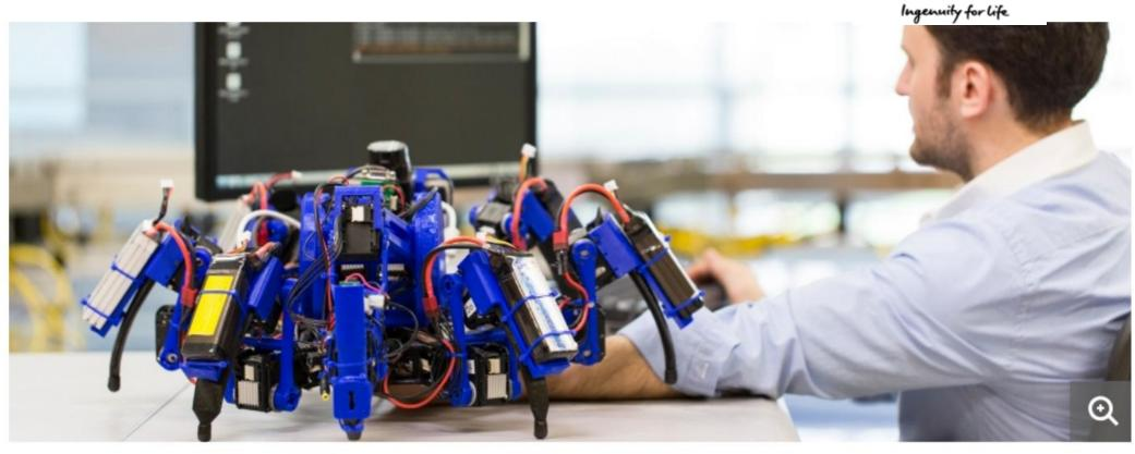
The next step in 3D printing could be something called mobile manufacturing. Siemens researchers in Princeton, New Jersey have developed prototype spider-like robots that can work collaboratively to print structures and surfaces, thus potentially accelerating production of large-scale, complex structures such as the fuselages of planes and the hulls of ships.
